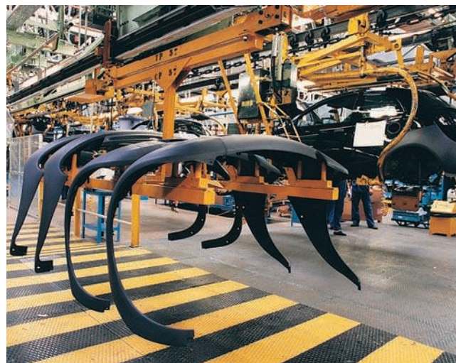
At Ford Motor Company's plant in Valencia, Spain, suppliers feed parts such as these bumpers just in time and in the right order directly to the assembly line.
